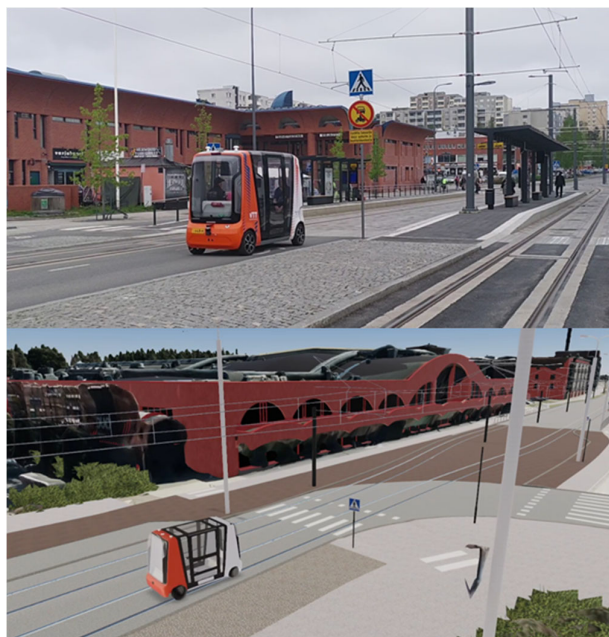
Figure 39. Autonomous vehicle in real world traffic (upper picture), and the respective virtualized autonomous vehicle in digital twin environment (lower picture).
