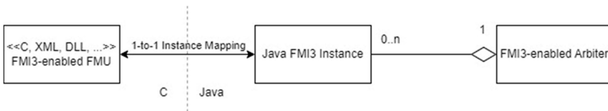
Figure 46: Concept for the support of FMI3 by the FERAL-based virtual evaluation platform.
