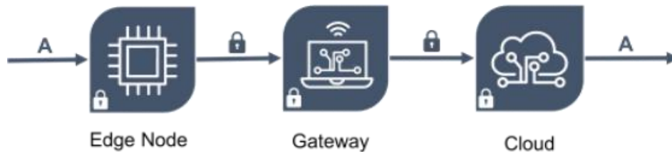
Figure 13: Data collection system in the project uses common IoT system architecture.
